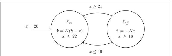
Figure 2.7: The hybrid automaton model of the thermostat
