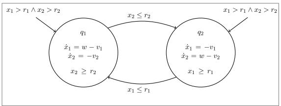
Figure 2.8: The hybrid automaton model of the water-level monitor
