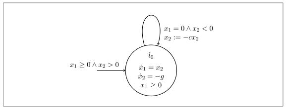
Figure 2.9: The hybrid automaton model of the bouncing ball
