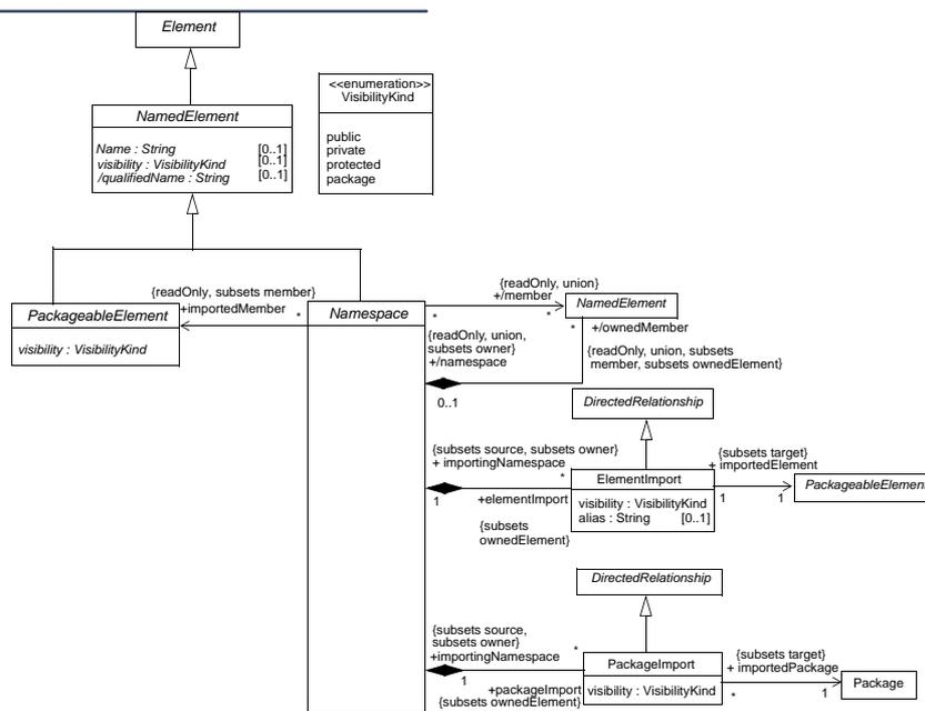
Figure 7.4 - Namespaces diagram of the Kernel package
