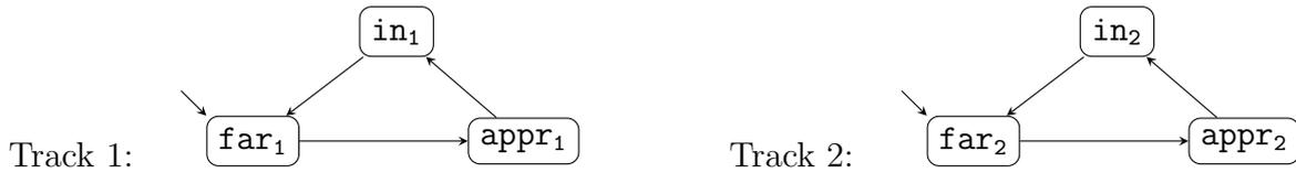
Describe a controller (in the form of a transition system) that controls the gate such that whenever a train is in the railroad crossing (state  $\text{in}_1$  or state  $\text{in}_2$ ), the gate is down (state **down**). Your controller may temporarily stop a train in the sense that a train may only move from  $\text{appr}_i$  to  $\text{in}_i$  if the controller agrees.
