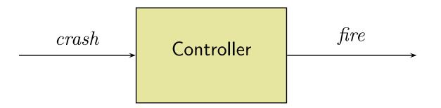
Requirement: "When a crash is detected, fire the airbag."
