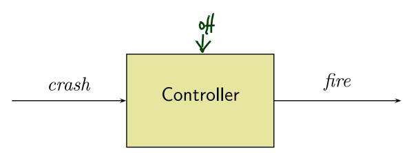
"When a crash is detected at time t, fire the airbag at  $t+300ms\pm\varepsilon$ ."
