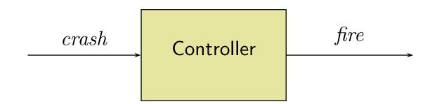
**Requirement**: "When a crash is detected, fire the airbag."
