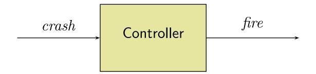
"When a crash is detected at time t, fire the airbag at  $t + 300 ms \pm \varepsilon$ ."
