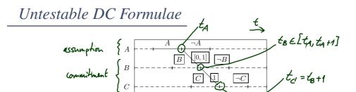
"Whenever we observe a change from A to  $\neg A$  at time  $t_A$ , the system has to produce a change from B to  $\neg B$  at some time  $t_B \in [t_A, t_A + 1]$  and a change from C to  $\neg C$  at time  $t_B + 1$ .
