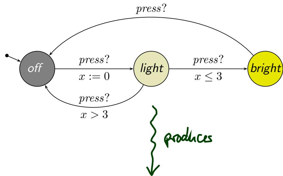
$$\xi = \langle off, 0 \rangle, 0 \xrightarrow{1} \langle off, 1 \rangle, 1 \\ \xrightarrow{\text{press?}} \langle light, 0 \rangle, 1 \xrightarrow{3} \langle light, 3 \rangle, 4 \\ \xrightarrow{\text{press?}} \langle bright, 3 \rangle, 4 \xrightarrow{\dots}$$
