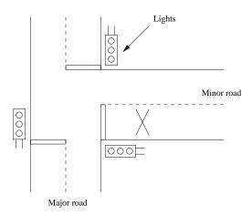
(a) First we ignore all timing issues involved and concentrate on the qualitative aspects of the behavior of the traffic lights. Model the above system as a network of timed automata, one for the minor-road lights, one for the major-road lights, and one for the car controller on the minor road.
