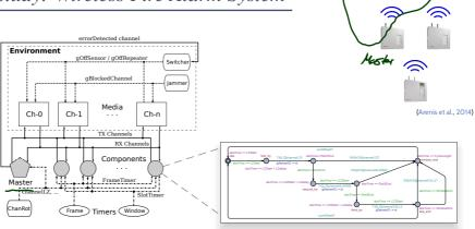
(R1) The loss of the ability of the system to transmit a signal from a component to the central unit is detected in less than 300 seconds [...].
