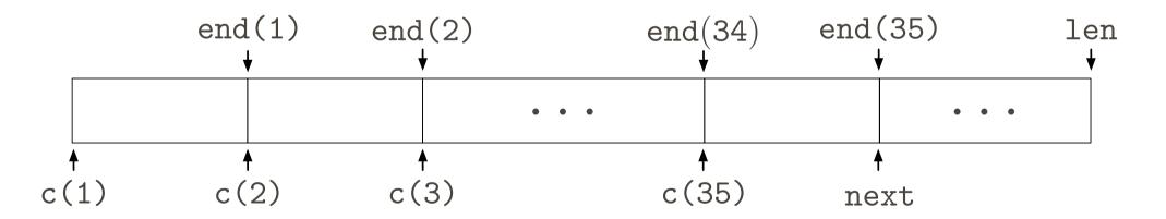
threads  $1, 2, \ldots, 35$ have acquired block of tasks have not yet started working
