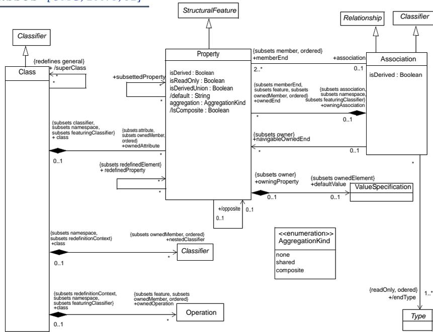
Figure 7.12 - Classes diagram of the Kernel package
