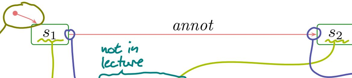
$annot ::= [ \underbrace{\langle event \rangle [ \cdot \langle event \rangle ]^*}_{\text{trigger}} \underbrace{[ \text{I} \langle guard \rangle \text{I} ]}_{\text{guard}} \underbrace{[ \text{/} \langle action \rangle ]}_{\text{action}} ]$
