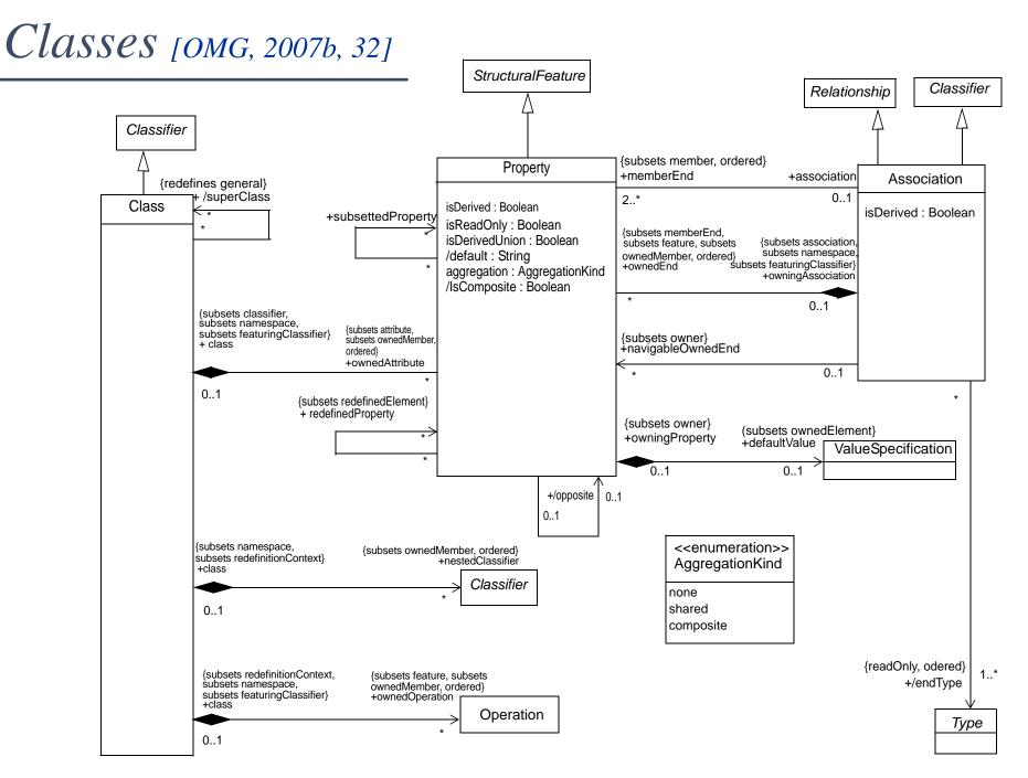
Figure 7.12 - Classes diagram of the Kernel package
