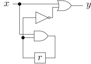
Provide the transition system of this hardware circuit. The states are the evaluations of the input  $x$  and the register  $r$ . The transitions represent the stepwise behavior of the circuit. The values of the input  $x$  change nondeterministically. The atomic propositions  $\{X, Y, R\}$  stand for  $x = 1$ ,  $y = 1$  and  $r = 1$ , respectively. Initially the register  $r$  has the value 1 (**true**).
