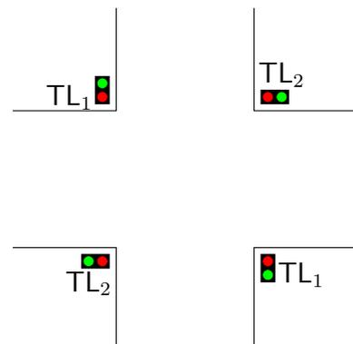
We model this system with two transition systems,  $TS_1$  and  $TS_2$ , for the traffic lights, one for each direction of the crossing. To avoid car crashes, these transition systems are connected via an arbiter that ensures only one traffic light can be green at a time.
